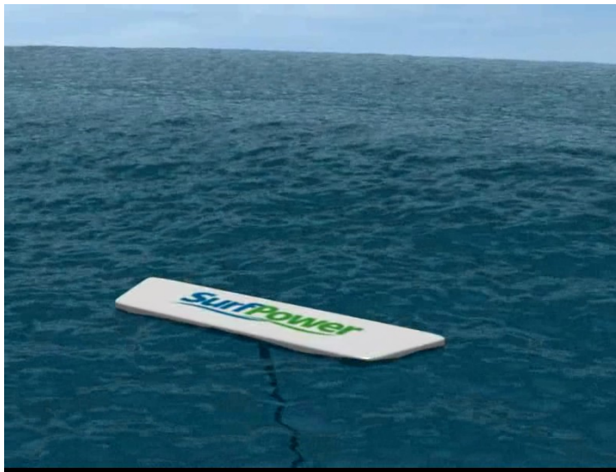
Figure 14: SurfPower device in 3.7 m, 11 s Airy waves
